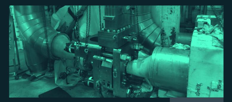
A platform operator in the Norwegian North Sea had a problem with a passing valve related to the second stage separator containing hydrocarbons at 90 bar (1300 psi) and 75 degrees C (165° F). From initial enquiry, Izomax designed, engineered and implemented a solution in just eight weeks, with no loss of productive time. The Izomax AOGV mechanical isolation tool was tested, certified and CE marked prior to mobilisation.
